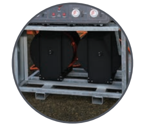
4 Umbilical reels, each for up to 100M
