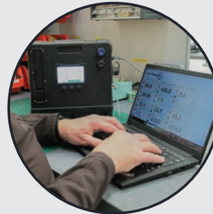
PC app and communication module for modifying settings
